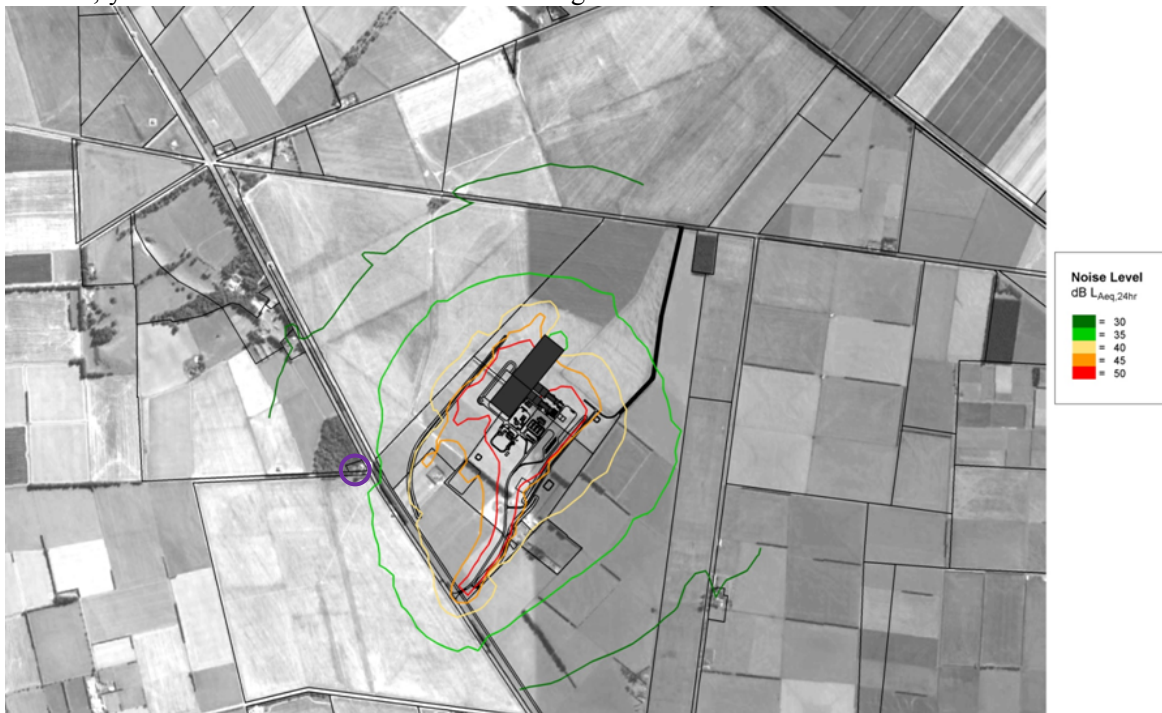
Figure 4 – Fonterra Darfield noise contours for stages 1 & 2 plus tanker shift change while loading rail.
